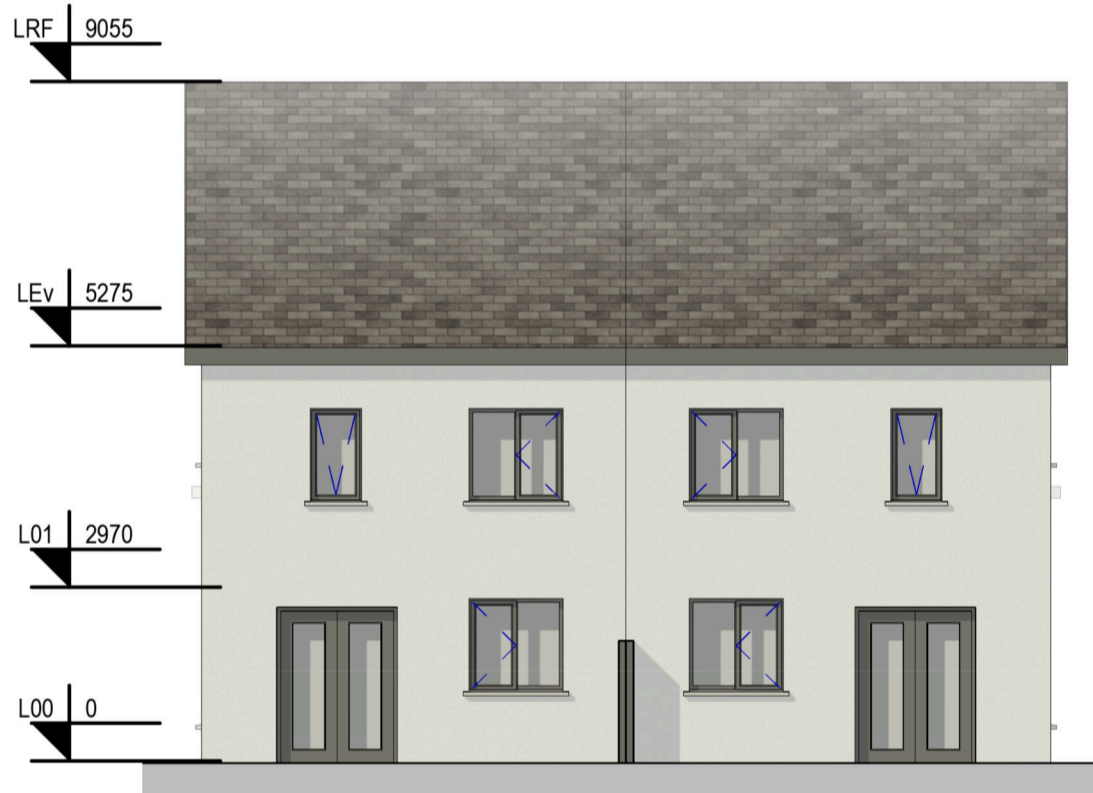
7: BHC1 Rear Elevation Scale - 1 : 100
