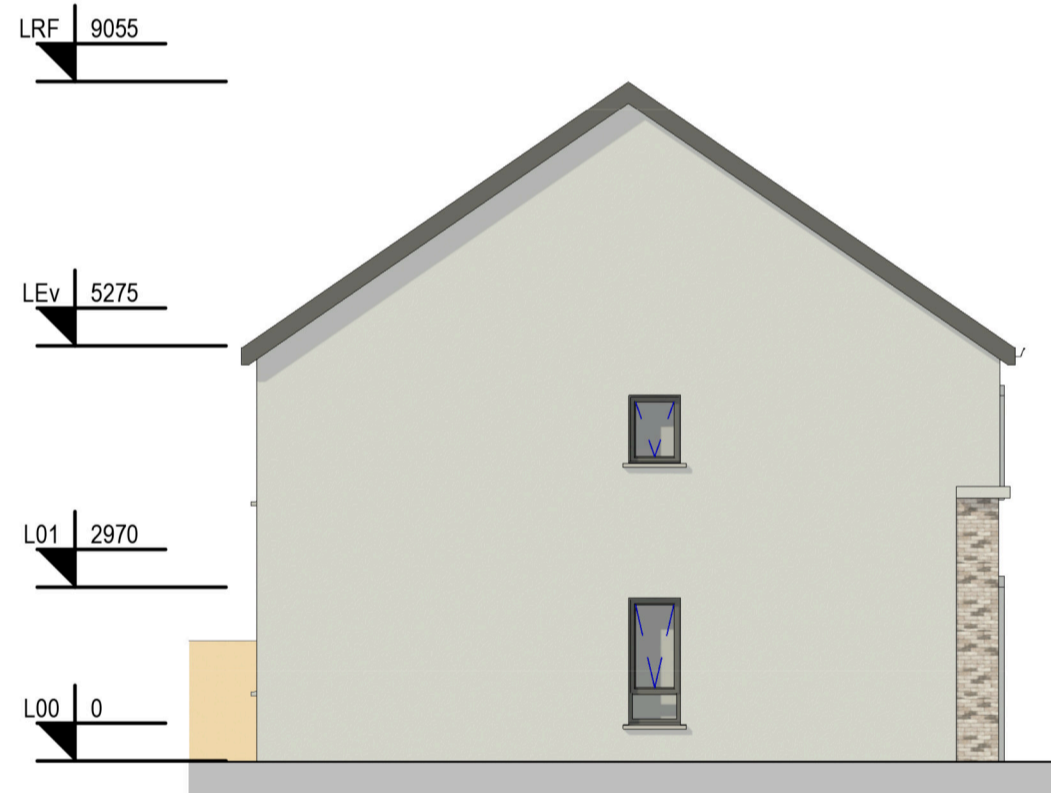
6: BHC1 Left Side Elevation Scale - 1 : 100
