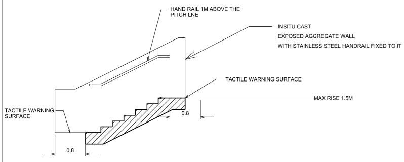
LD 12 EXPOSED AGGREGATE INSITU CAST CONCRETE STEPS
