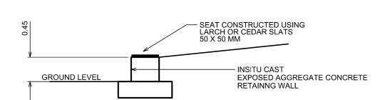
LD 13 LOW RETAINING WALL / SEAT MAX HEIGHT 450 MM FOR CONSTRUCTION DETAILS SEE CIVIL ENGINEERS DETAILS
